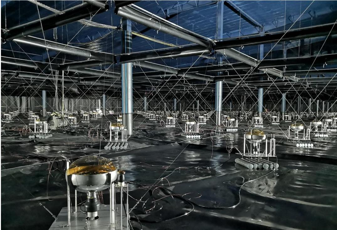
20-inch PMTs installed in LHAASO
