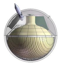
Figure 2: Optical module design schematic. A 20-inch PMT encapsulated inside a 23-inch glass sphere.
